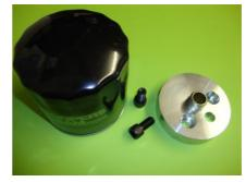
completely, including the bowl and filter. Clean the engine block where the filter head was located and remove the old gasket. Ensure that the mating surface is clean and dry.
